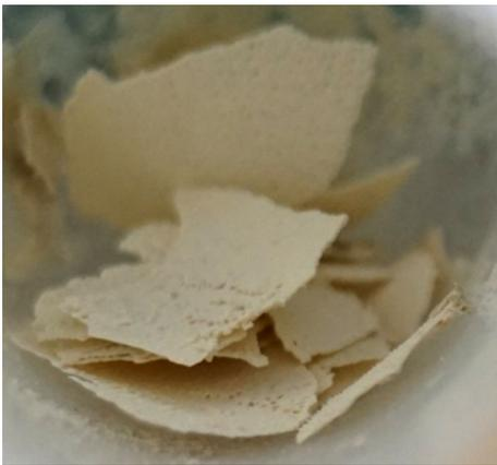
**Fig. 3** Calcium carbonate crystals precipitated after mixing *Staphylococcus* sp. IR-103 suspension grown in YN medium with cementation solution (1:1 v/v) for 15 days at room temperature
