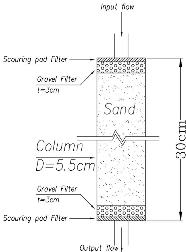
Fig. 1 Schematic details of column packed with Anzali’s sandy soil
