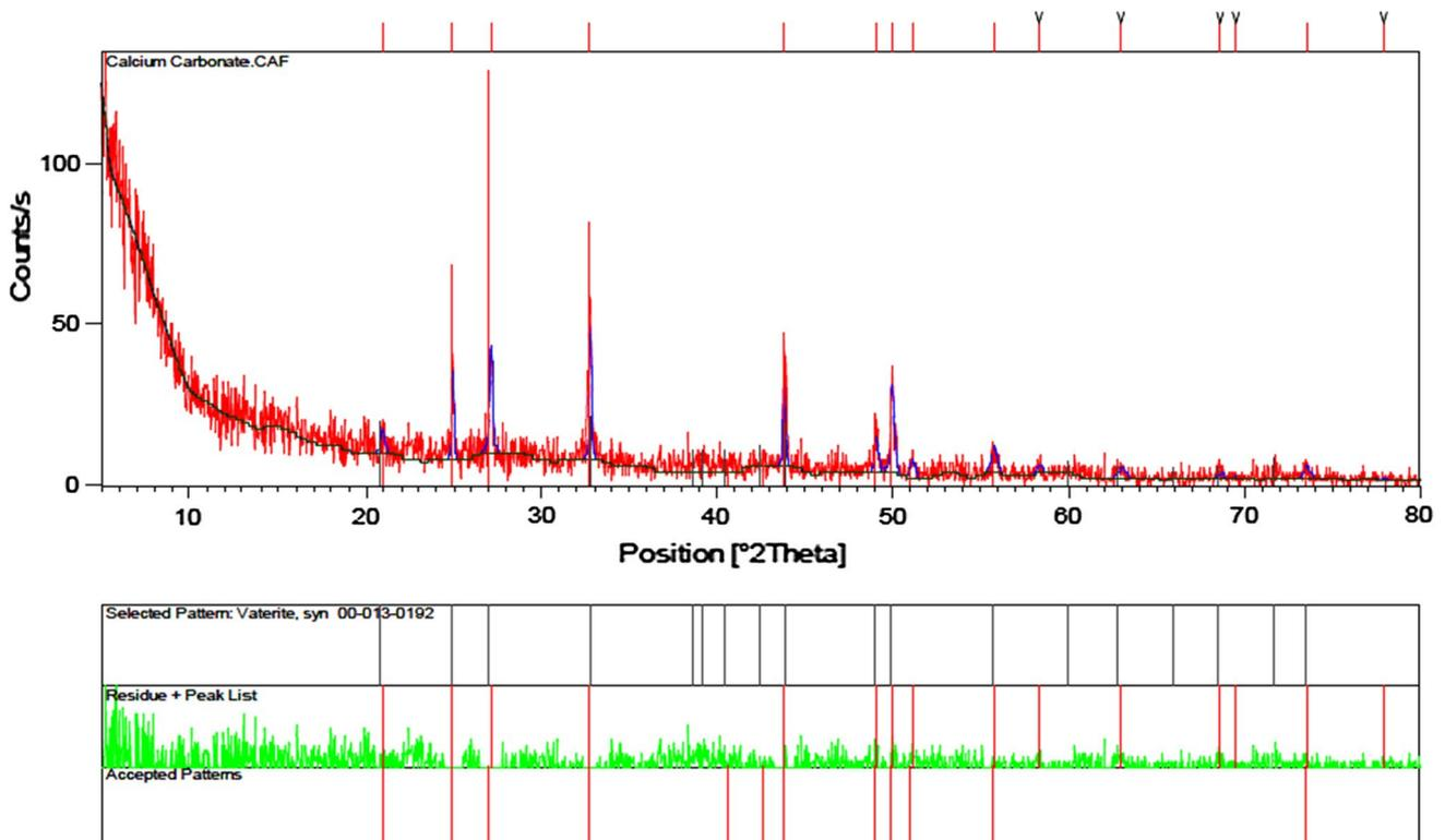
Fig. 6 The XRD pattern for calcium carbonate precipitated by the biocementation reaction demonstrates that the most dominant mineral composition is that of vaterite
