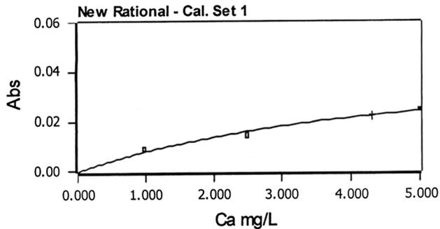
Fig. 5 AAS graph of calcium carbonate precipitated during the biocementation reaction by *Staphylococcus* sp. IR-103
