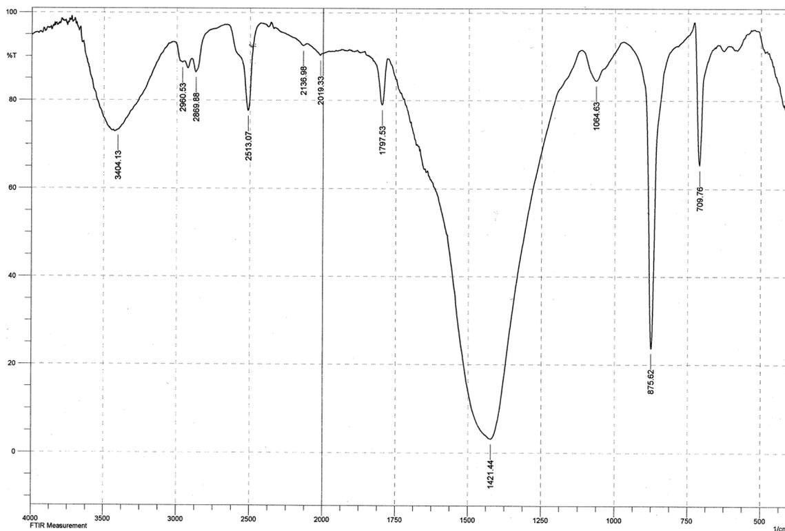
**Fig. 4** FTIR spectrum of calcium carbonate precipitated by *Staphylococcus* sp. IR-103 grown on YN medium
