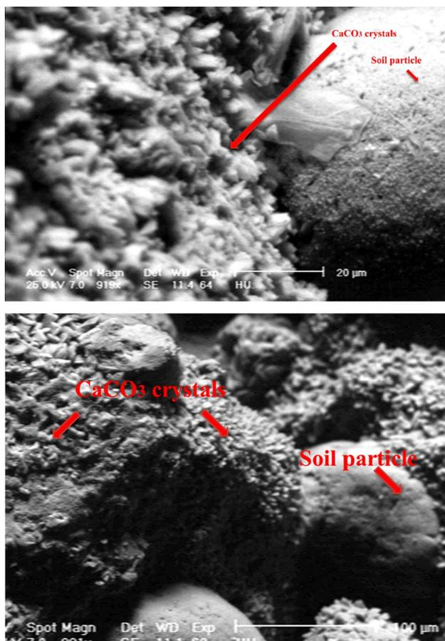
**Fig. 7** SEM micrograph of biocemented sandy soil. The biotreated column samples were cut into small sections, coated with gold and then scanned. CaCO<sub>3</sub> crystals formed between the sandy soil particles and on their surfaces are clearly observed
